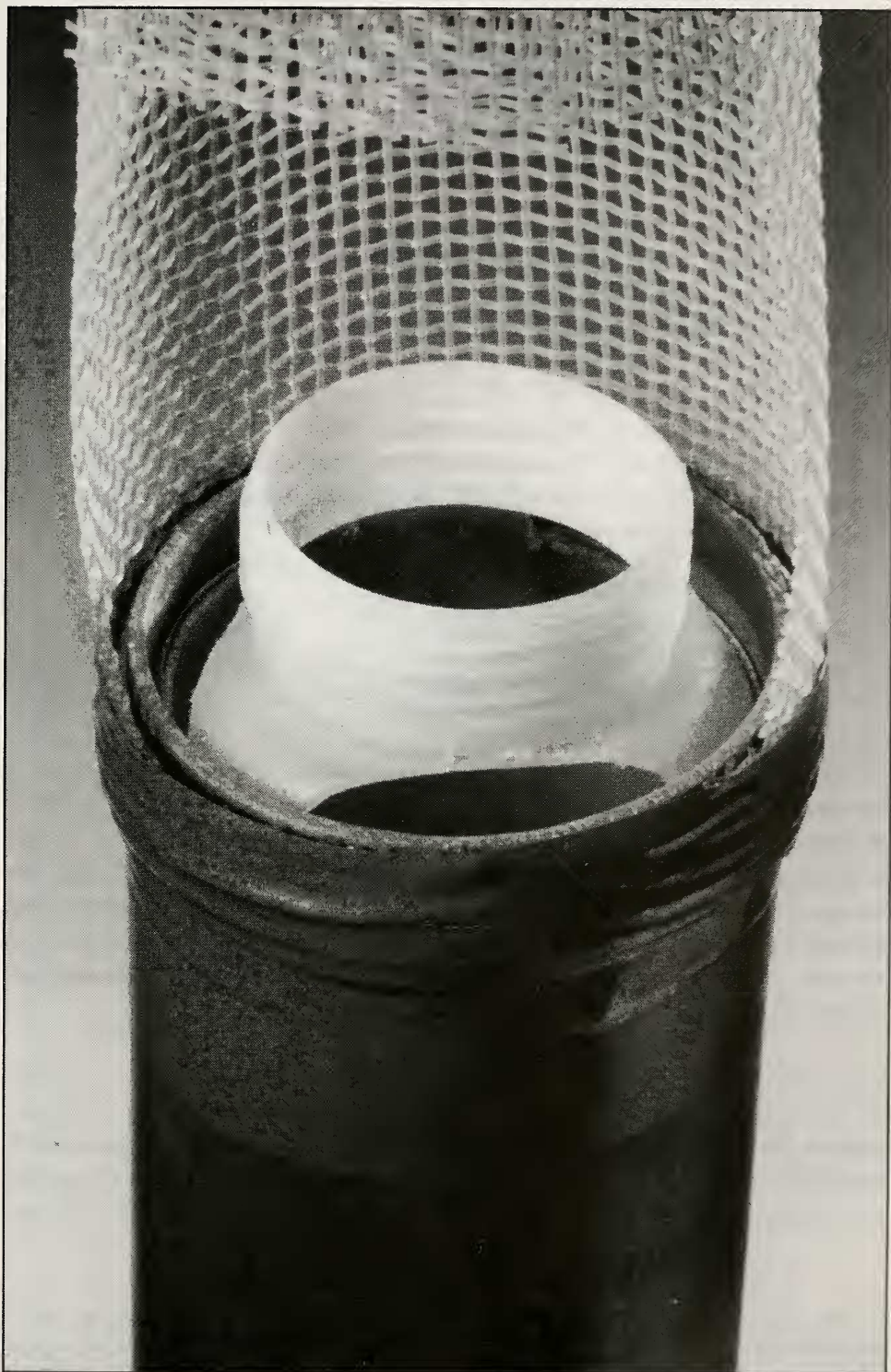
The photograph shows the region of the trap at the junction of the netting and the rigid pipe. A piece of the netting has been cut away to show how the collecting bottle sits neatly in the rigid pipe at the bottom of the trap.
